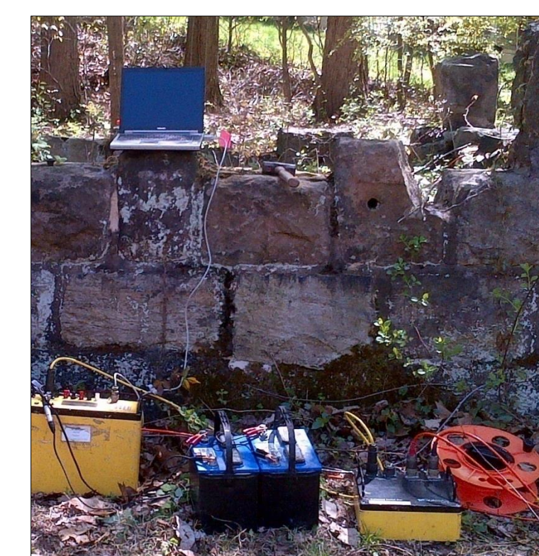
Figure 4: 3-D Resistivity Survey equipment
